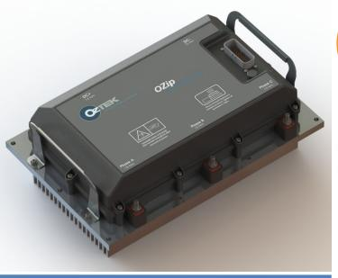
OZip IPMs are designed and qualified for demanding environments. They utilize ruggedized construction throughout, and feature an encapsulated planar DC link with polypropylene film capacitors, and automotive grade components with generous deratings. All OZip IPMs are environmentally stress screened to further ensure high reliability.
