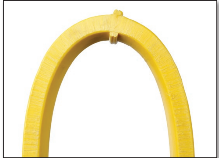
BEND BACK TESTING - NO GAPS OR VOIDS (See Figure 1)
