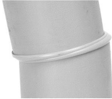
Figure 3. UNACCEPTABLE APPEARANCE – Mitered Joint – Improper ‘High-Low’ Pipe Alignment
