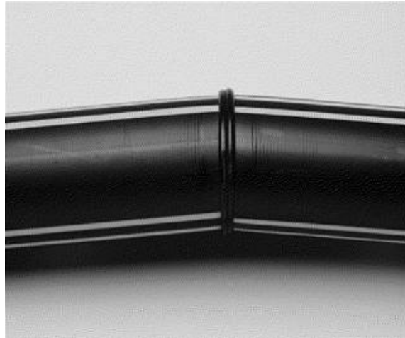
Figure 4. UNACCEPTABLE APPEARANCE – Unintentional Mitered Joint – Improper Alignment in Fusion Machine
