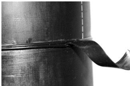
Figure 5. UNACCEPTABLE APPEARANCE – Contamination in Joint
