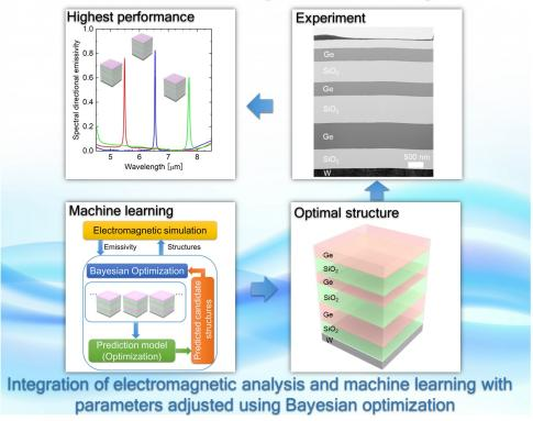
Schematic diagram showing the materials informatics method combining machine learning and the calculation of thermal emission properties and experiments conducted to verify the performance of fabricated materials
