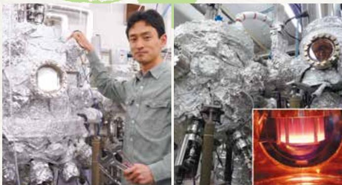
This is a molecular beam epitaxy system (MBE system) that is used for producing high-quality crystal thin films. This device allows us to create an ultrahigh vacuum up to  $10^{-8}$  Pa. Given that the vacuum level near the International Space Station is about  $10^{-6}$  Pa at an altitude of about 400 km, you can see that it is possible to artificially create a very high vacuum in MBE. MBE systems are expensive and cost approximately between 50 and 100 million yen.
