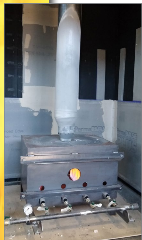
Testing a wood-burning stove heat shield.
