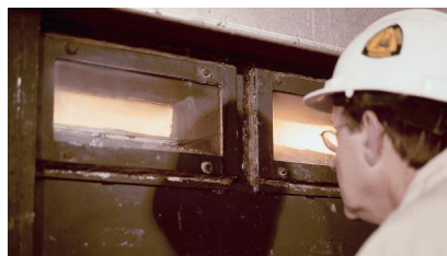
An associate looks into the Steiner Tunnel test furnace.
