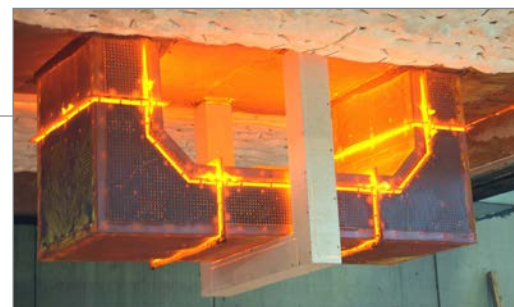
Eureka! How a winning sample looks after the 3-hour fire-endurance test.
