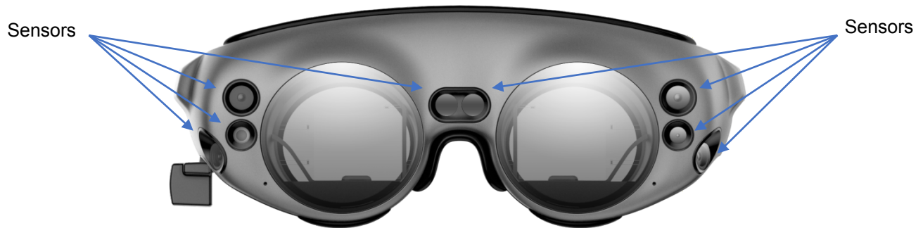
Figure 2 2– Sensors on HMD
