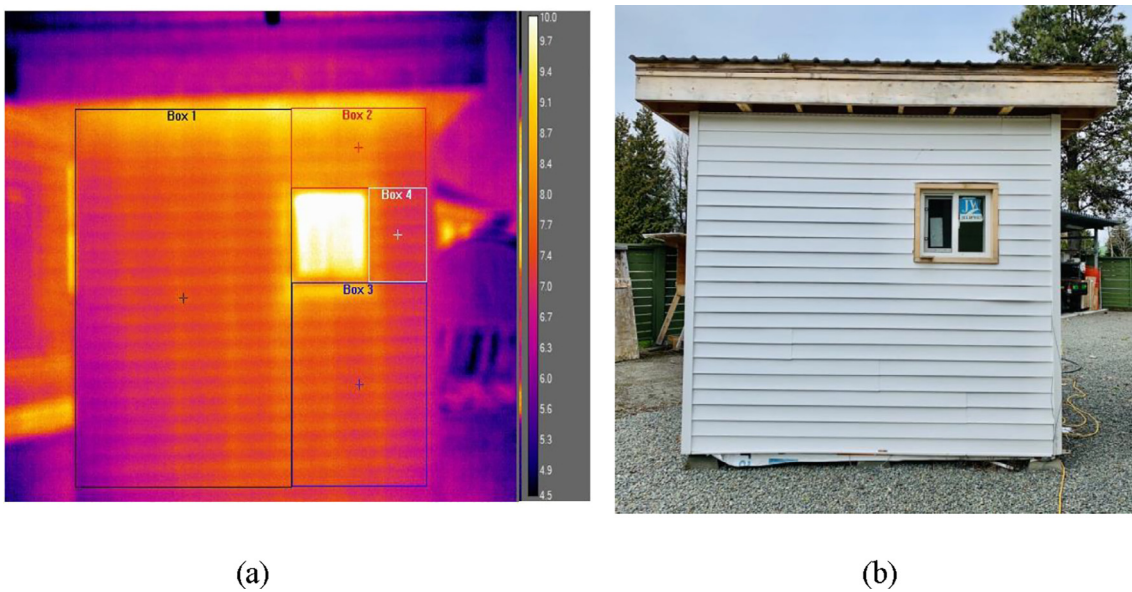
Fig. 8. Selection of region of interests (ROIs) to estimate U-value of W1: (a) thermal image; and (b) photograph.
