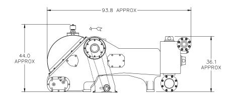
Note: All installations must contain a pressure relief valve in the discharge line near the pump.
