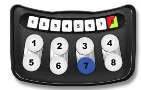
2 LED 8 will be flashing red and green to indicate entering the programming menu.
