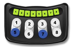
1 Press and hold 5 and 7 while turning the wheelchair ON.
